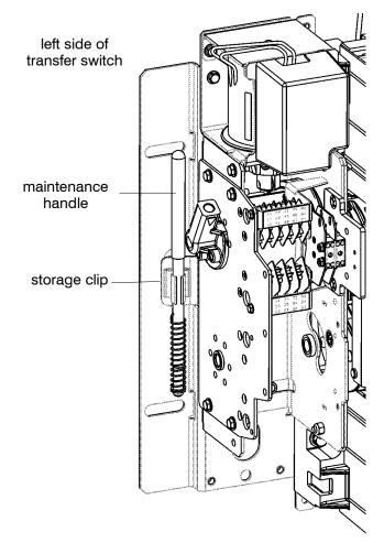
Figure 1-2. Maintenance handle and its storage clips.
